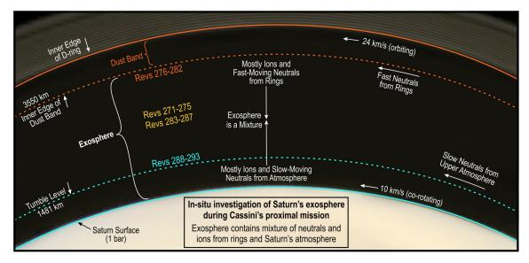
Figure 3-18. Geometry of Cassini's Grand Finale orbits. Left panel: A schematic drawing showing the altitude coverage of the orbits (revs) during the Grand Finale phase of the Cassini mission from a polar perspective. The region is bounded above by the D-ring and below by the 1 bar pressure level of Saturn's atmosphere. From Waite et al. [2018].
