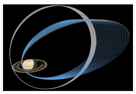
Figure 3-3. Cassini's 20 Ring Grazing (gray) and Grand Finale (blue) orbits. The last half-orbit (orange) took Cassini into Saturn's atmosphere for vaporization.
